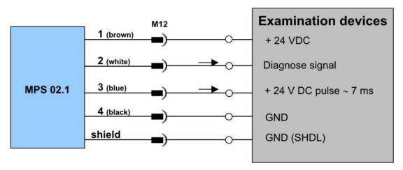
After connecting the MPS 02.1 and the power cable to your system, the sensor is ready for operation.
