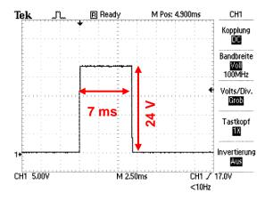
The standard signal is a square pulse with amplitude of 24 V and a pulse length of 7 ms at a sensor operating voltage of 24 V DC.
